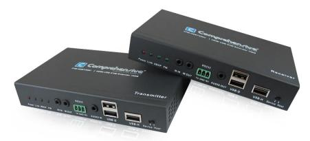
features that include 4K2K@60Hz (YCbCr 4:2:0) video, audio, control (IR or RS-232), Power over Ethernet (PoE) and an Ethernet connection. The Transmitter or Receiver can be powered by the PoE function using one power cable. In addition, the Extender set can support the connection of USB host and two USB devices that can control the source from the Sink side – 330 feet away. And, the Extender is HDCP 2.2 compliant for protected content streaming.
