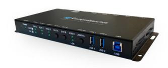
Comprehensive's CSW-302PSMC is a highly flexible 3x2 matrix switcher designed to meet the demands of various environments requiring versatility in inputs, outputs, and control. It offers the two most used video input interfaces, HDMI and USB-C, along with two HDMI outputs, ensuring excellent source compatibility and flexibility. This unit is HDCP 2.2 compliant and supports resolutions up to 4K@60Hz (4:4:4, 8-bit), delivering high-quality visuals.
